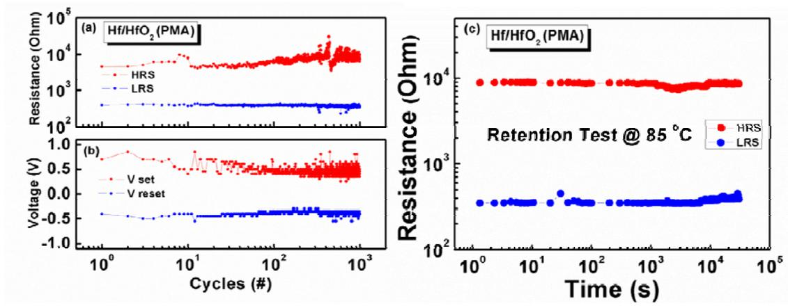
**Figure 6.** The 10<sup>3</sup> stable endurance cycles of the Pt/Hf/HfO<sub>2</sub>/TiN device: (a) HRS and LRS. (b) V<sub>set</sub> and V<sub>reset</sub>. (c) Data retention characteristics at 85 °C under 100mV stress.
