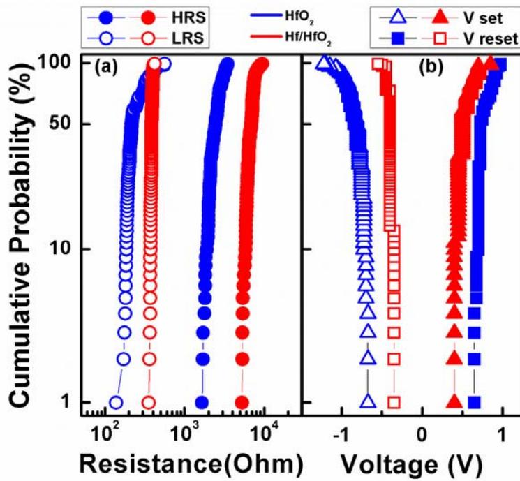
**Figure 5.** Statistical distribution of resistive switching parameters during 100 continuous cycles in both Pt/HfO<sub>2</sub>/TiN and Pt/Hf/HfO<sub>2</sub>/TiN devices. (a) HRS and LRS. (b) V<sub>set</sub> and V<sub>reset</sub>.
