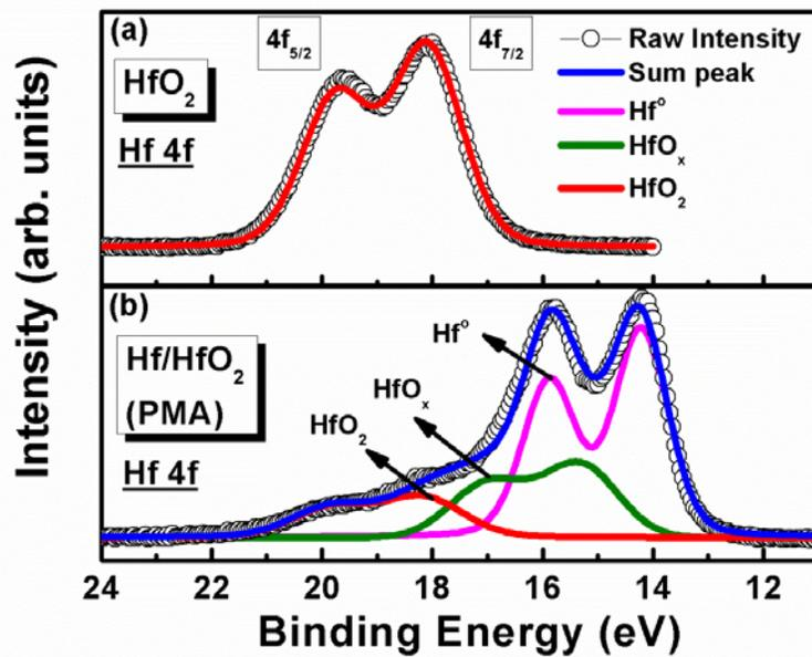
**Figure 3.** XPS spectra of Hf 4f core levels: (a) the HfO<sub>2</sub> thin film. (b) Interface between Hf/HfO<sub>2</sub>.
