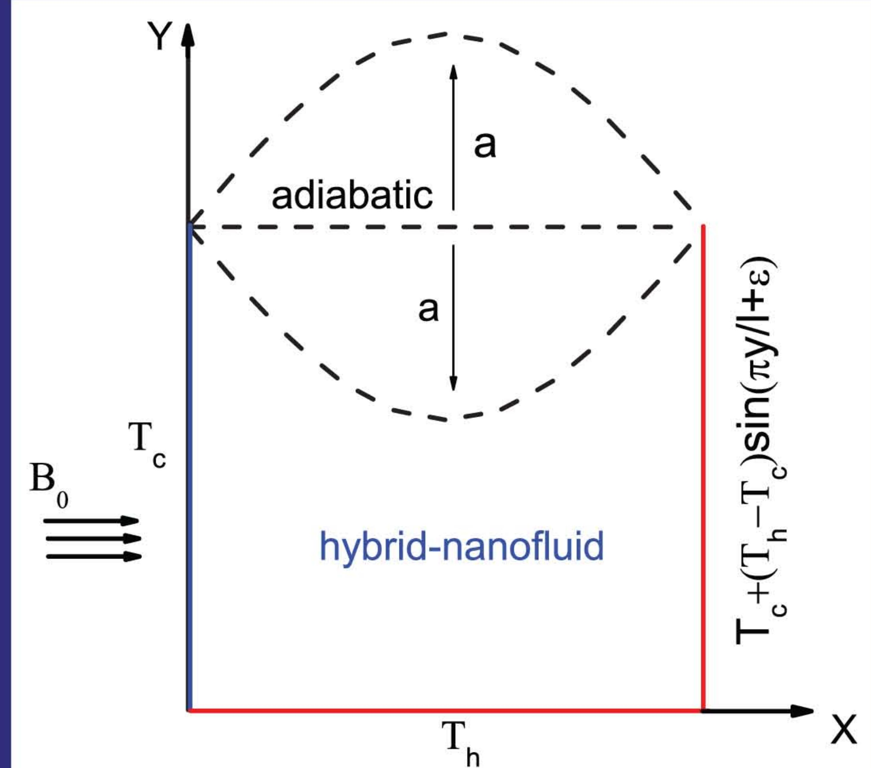
*On the cover:* MHD natural convection of a hybrid nanofluid in a curved enclosure with various amplitudes. Courtesy: Parveen et al. JON 10(3) 2021
