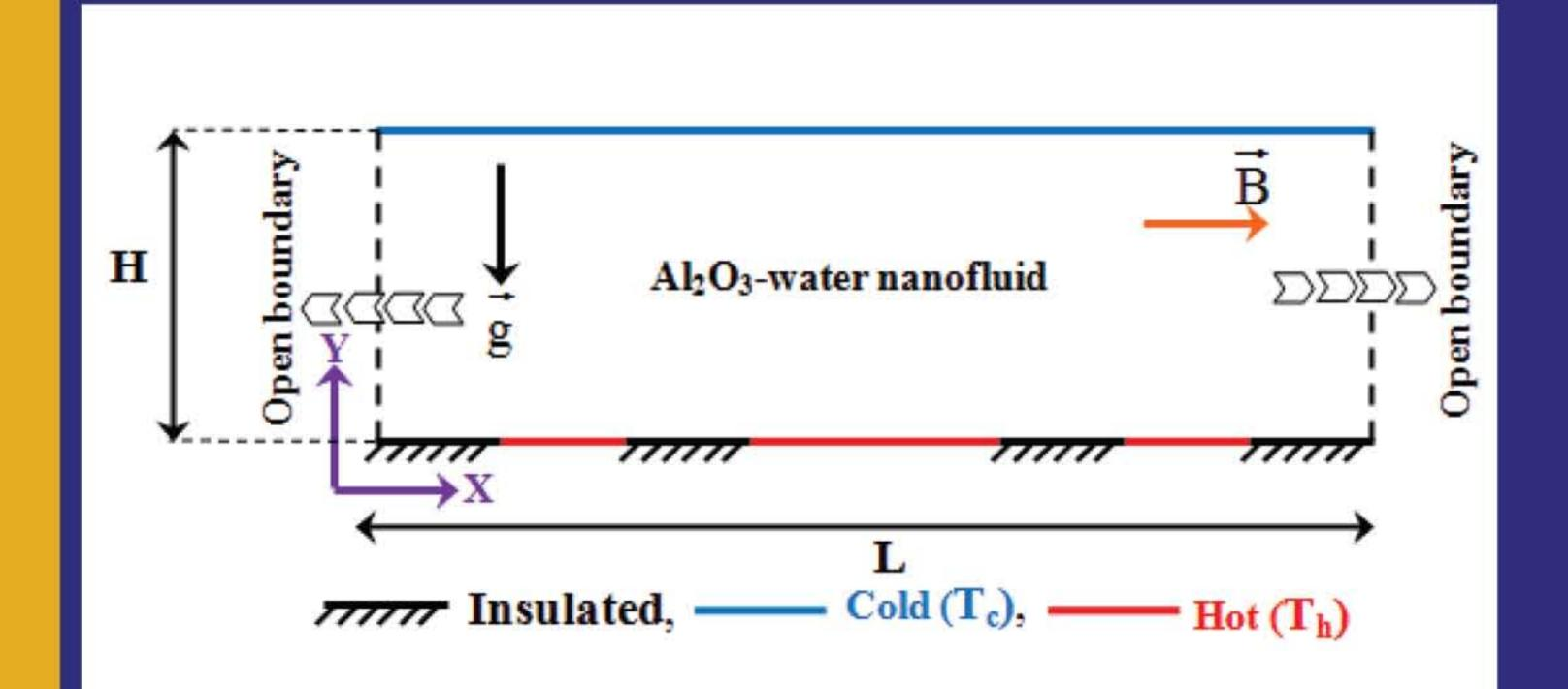
On the cover: Schematic representation of the studied configuration. Courtesy: Ferhi et al. JON 11(4) 2022
