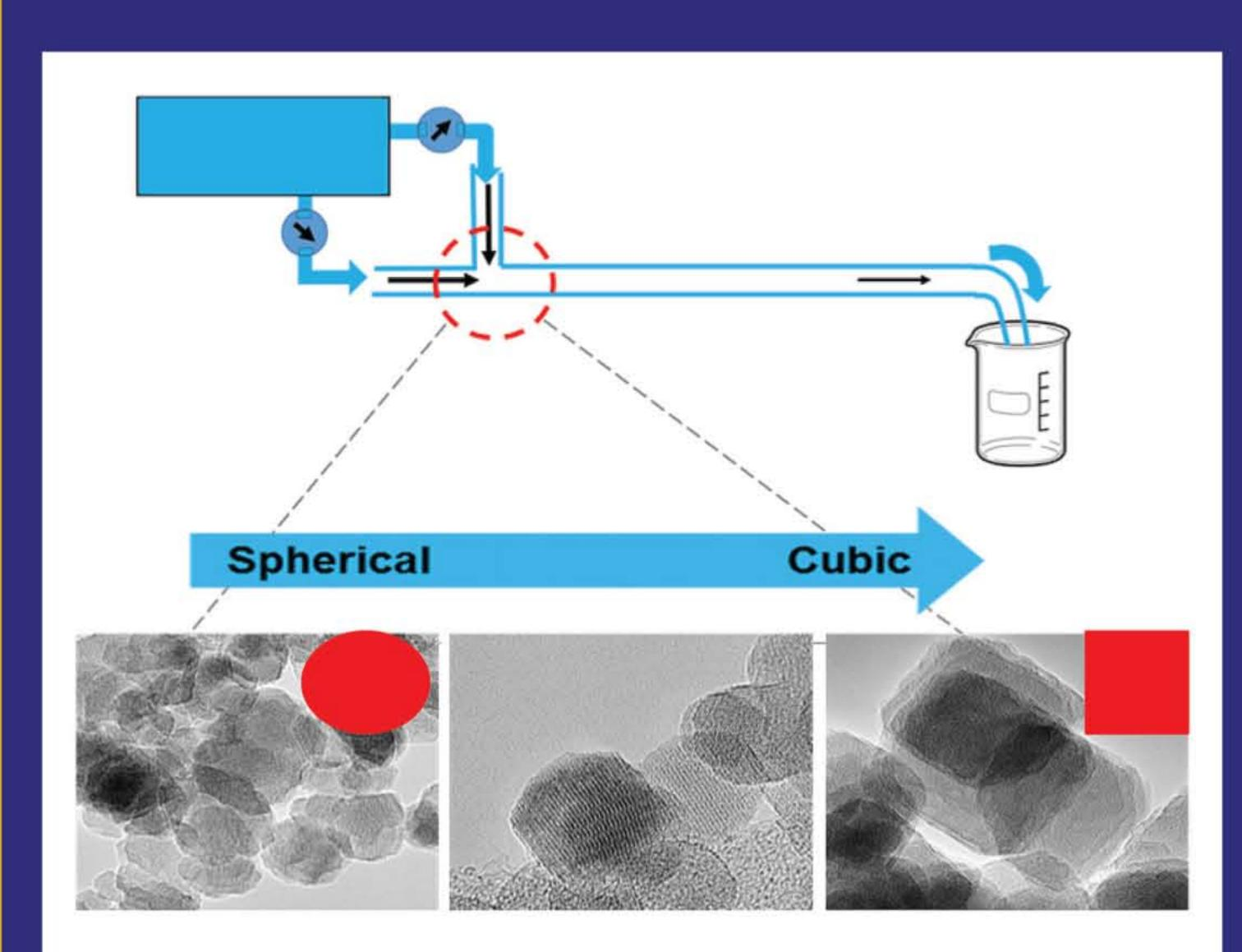
On the cover: Schematic illustration of the experimental setup for the magnetic nanoparticle synthesis in a microchannel with size and shape variation (Courtesy: A. Ray et al.) JON 5 (6) 2016.
