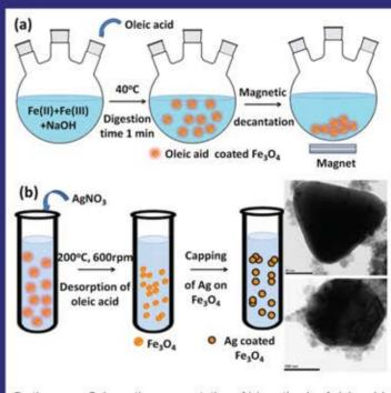
On the cover: Schematic representation of (a) synthesis of oleic acid coated Fe<sub>3</sub>O<sub>4</sub> using co-precipitation and (b) Ag coated Fe<sub>3</sub>O<sub>4</sub> by microwave assisted synthesis (Courtesy: C. Anushree et al.) JON 6 (1) 2017.
