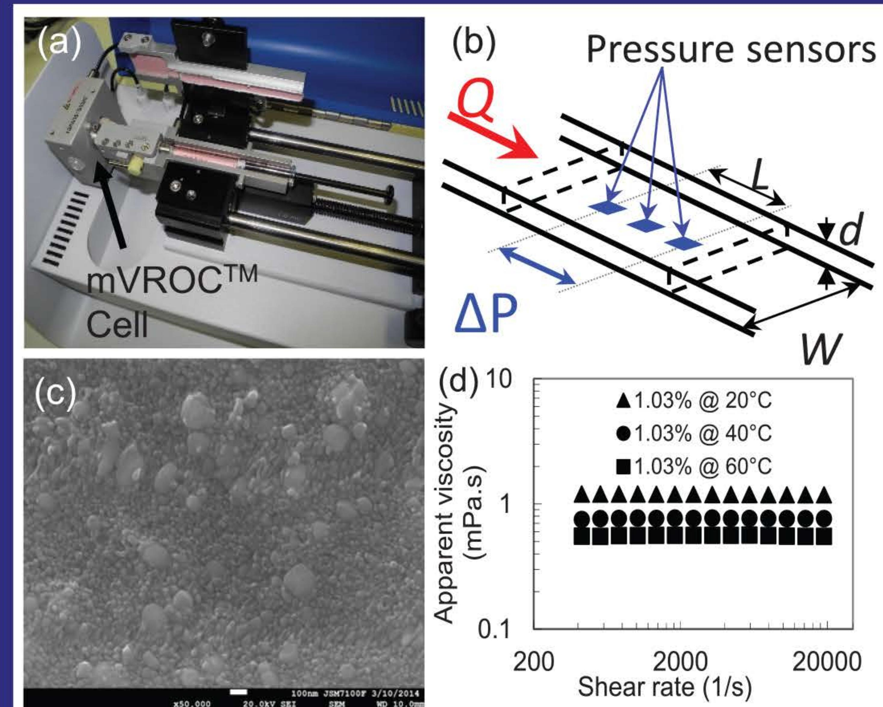
On the cover: (a) Photograph of mVROC™ and microfluidic sensor
