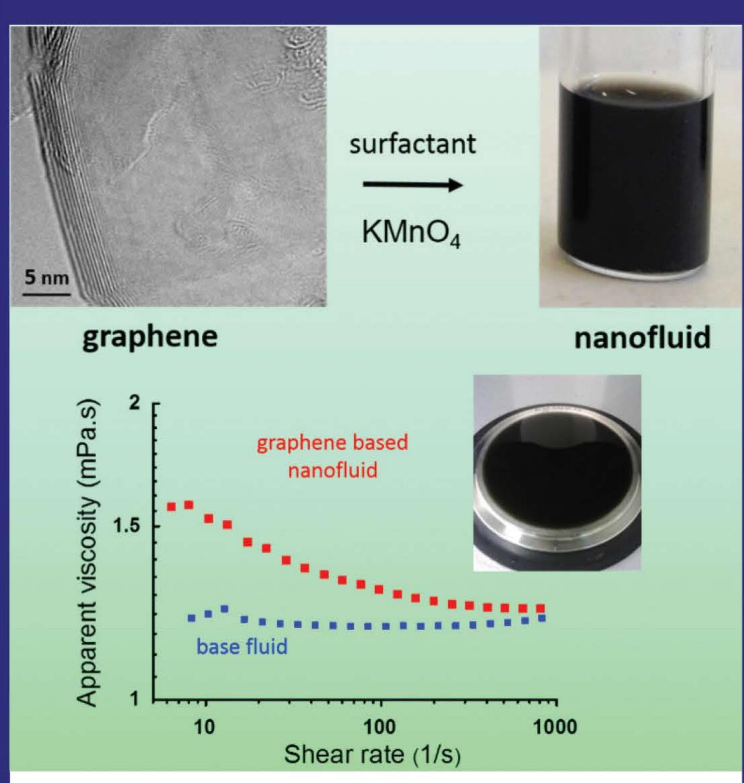
On the cover: Combination of non-covalent and low level covalent functionalization for the preparation of stable graphene-based nanofluids under static and dynamic conditions (Courtesy: Brigitte Vigolo) JON, 6(3) 2017
