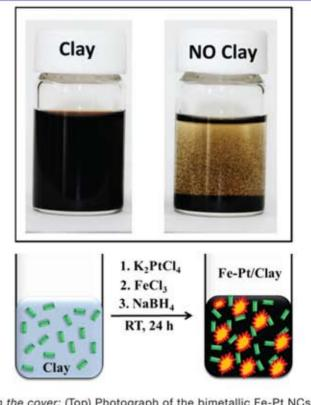
On the cover: (Top) Photograph of the bimetallic Fe-Pt NCs synthesized in the presence and absence of the clay under similar synthetic conditions (bottom) Synthesis of bimetallic Fe-Pt/clay nanocomposite material. (Courtesy: Dharmesh Varad) JON 6 (6) 2017.
