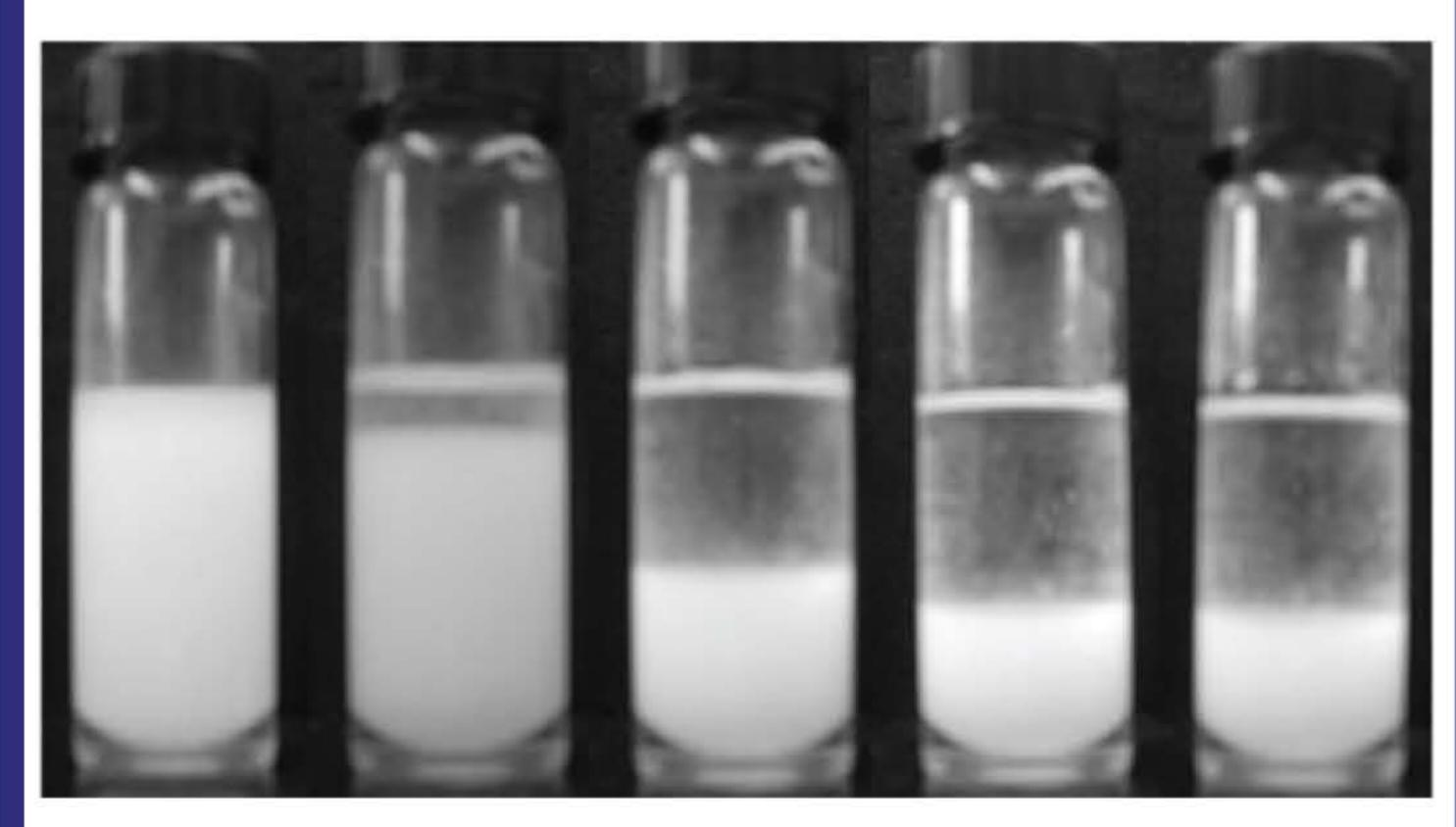
On the cover: (Top) Schematic of sequential addition of dispersed phase leading to catastrophic phase inversion. (bottom) Emulsions prepared using hydrophobic nanoparticles as a lone stabilizer. For more technical details, see *Rajinder Pal and Varun Malhotra*, pp. 300–308 of this issue.
