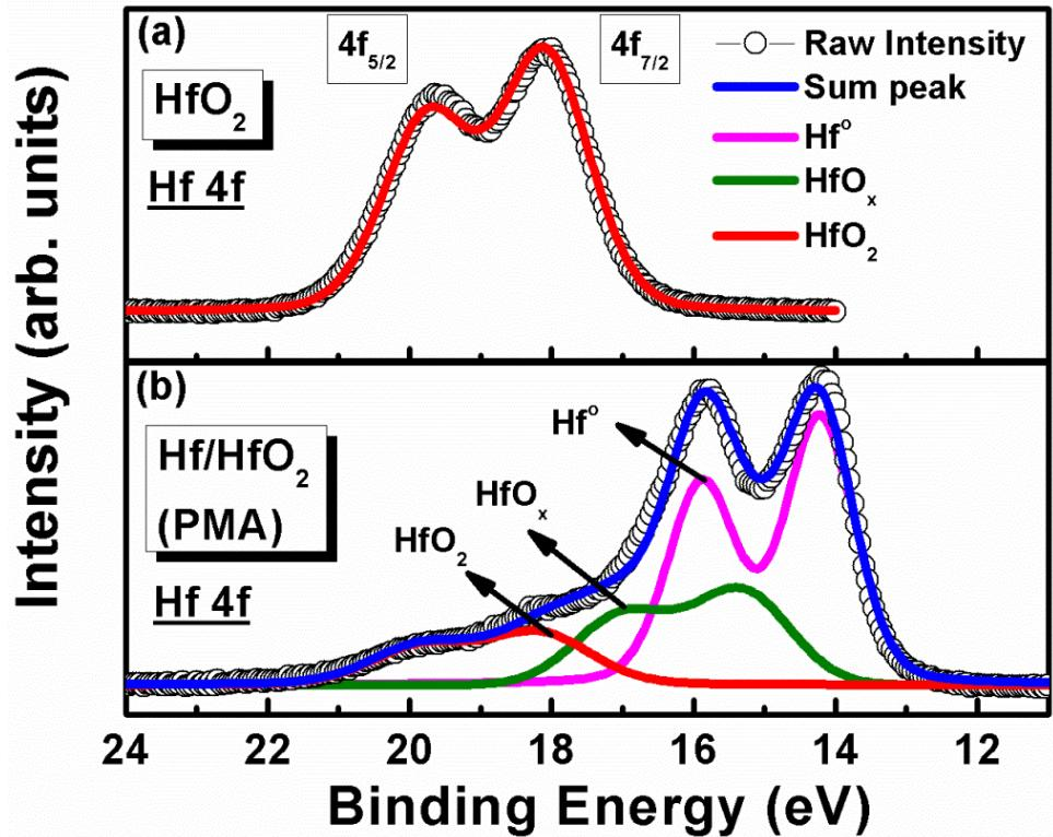
**Figure 3.** XPS spectra of Hf 4f core levels: (a) the HfO<sub>2</sub> thin film. (b) Interface between Hf/HfO<sub>2</sub>.
