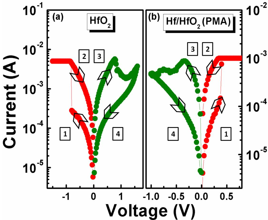
**Figure 1.** Reverse polarity operation in resistive switching between Pt/HfO<sub>2</sub>/TiN and Pt/Hf/HfO<sub>2</sub>/TiN devices.
