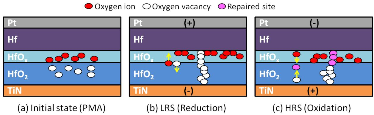
**Figure 4.** Possible scenarios of switching mechanisms for the Pt/Hf/HfO<sub>2</sub>/TiN device with positive-bias or negative-bias voltage.
