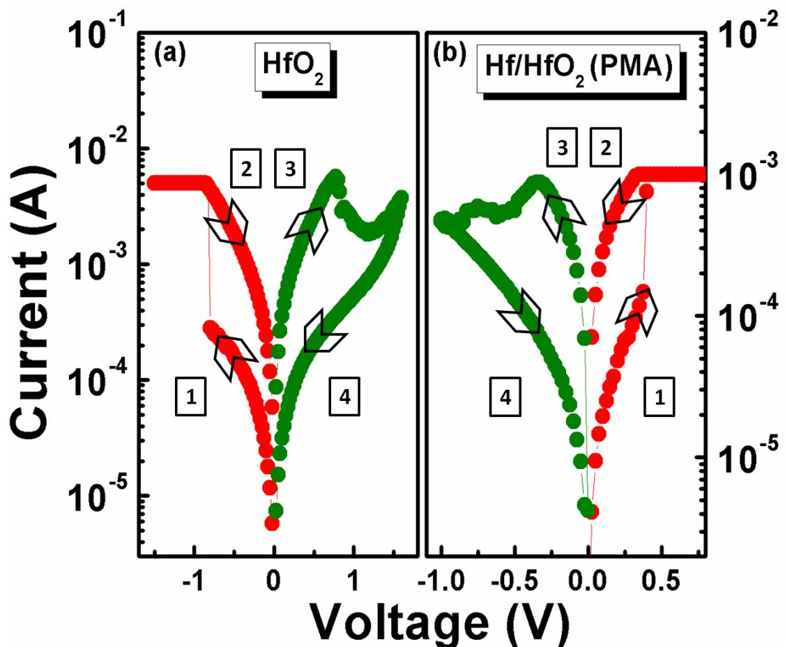
**Figure 1.** Reverse polarity operation in resistive switching between Pt/ $\text{HfO}_2$ /TiN and
