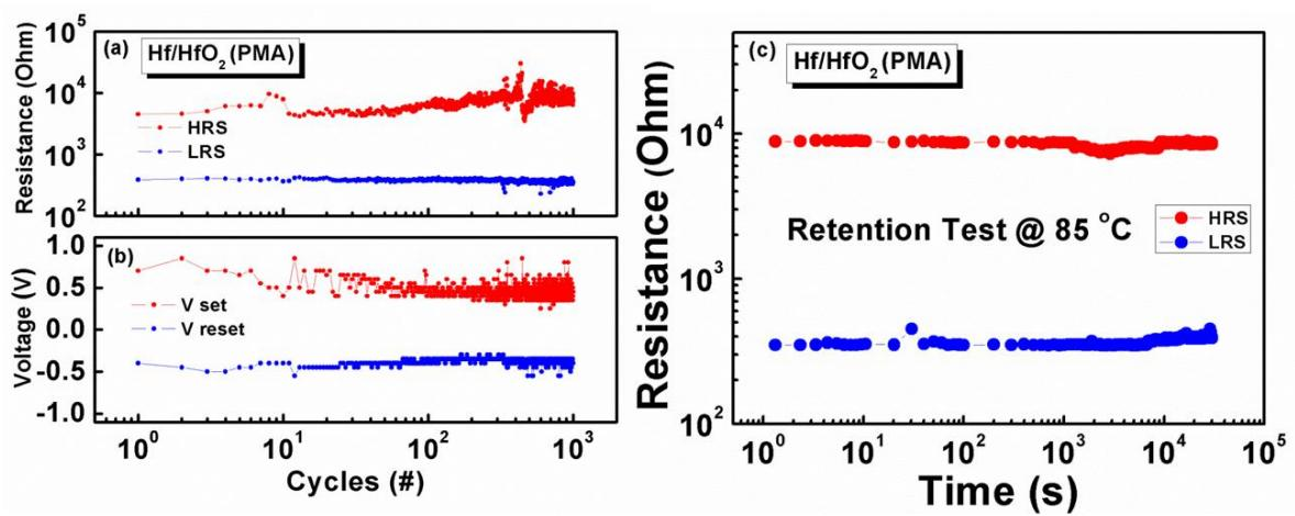
**Figure 6.** The  $10^3$  stable endurance cycles of the Pt/Hf/HfO<sub>2</sub>/TiN device: (a) HRS and LRS. (b) V<sub>set</sub> and V<sub>reset</sub>. (c) Data retention characteristics at 85 °C under 100mV stress.
